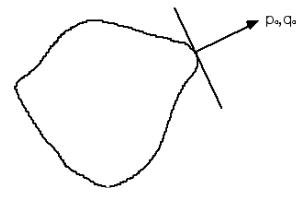
The surface normal can be read directly off the image if the boundary contours are known. But we have a problem, at smooth occluding bounding contours,  $p_o$  and  $q_o$  (the spatial rates of change of the surface depth away from the viewpoint) are infinite. And if the bounding contours are not smooth, but sharp, the surface normal is not defined there.
